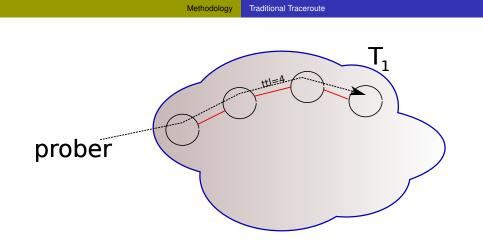
... continuing until finished with  $T_1$  (reach destination or gap limit). Prober must maintain state, while traffic is concentrated on *prober*  $\rightsquigarrow$   $T_1$  path
