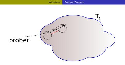
Traditional traceroute sends probes with incrementing TTL to destination  $T_1$
