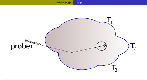
In contrast, Yarrp iterates through randomly permuted < *Target*, *TTL* > pairs
